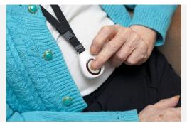
Commonly, a telecare alarm trigger is worn on the body, usually around the neck, or on the wrist. The person presses the button on the trigger to get help, especially if they fall and can't get up. When the TCP receives an alarm, they can talk to the person through a speaker. Many other types of telecare and telehealth devices are also available – go to 'Find TEC Services' at <a href="https://www.tsa-voice.org.uk/">https://www.tsa-voice.org.uk/</a>.
