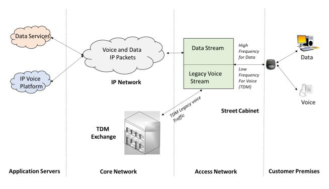
Figure 1 – An example of TDM and IP network current architecture
