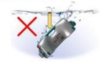
The Raizer must NOT be immersed in water
